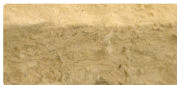
mineral wool (reduces heat loss & noise levels)
